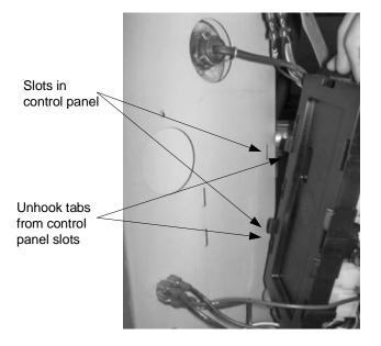
Step 2. Tilt control panel to the right and slide control hook tabs from slots in control panel.
